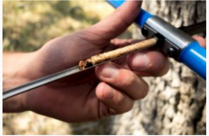
Pencil-like tree-ring cores are collected non-destructively using a Swedish increment borer in May, 2014. (Daniel Griffin/University of Minnesota)
